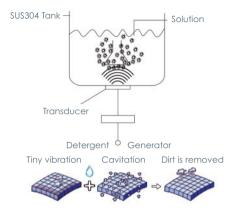
**Ultrasonic cleaning** is based on the cavitation effect caused by the vibration of high frequency ultrasonic waves in the liquid. Microscopic bubbles are formed. These implode causing the cavitation which create an intense scrubbing action on the surface of the item being cleaned. The bubbles are small enough to penetrate microscopic crevices, cleaning them thoroughly and consistently.
